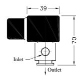
737641 Solenoid Valve 24VDC x <sup>3</sup>/<sub>64</sub>" Orifice <u>Material</u> : Nickle Plated Brass Body <u>Ports</u> : <sup>1</sup>/<sub>8</sub>" BSPT Female <u>Protection Rating</u> : IP65 Weatherproof Housing <u>Power Rating</u> : 24VDC 9W
